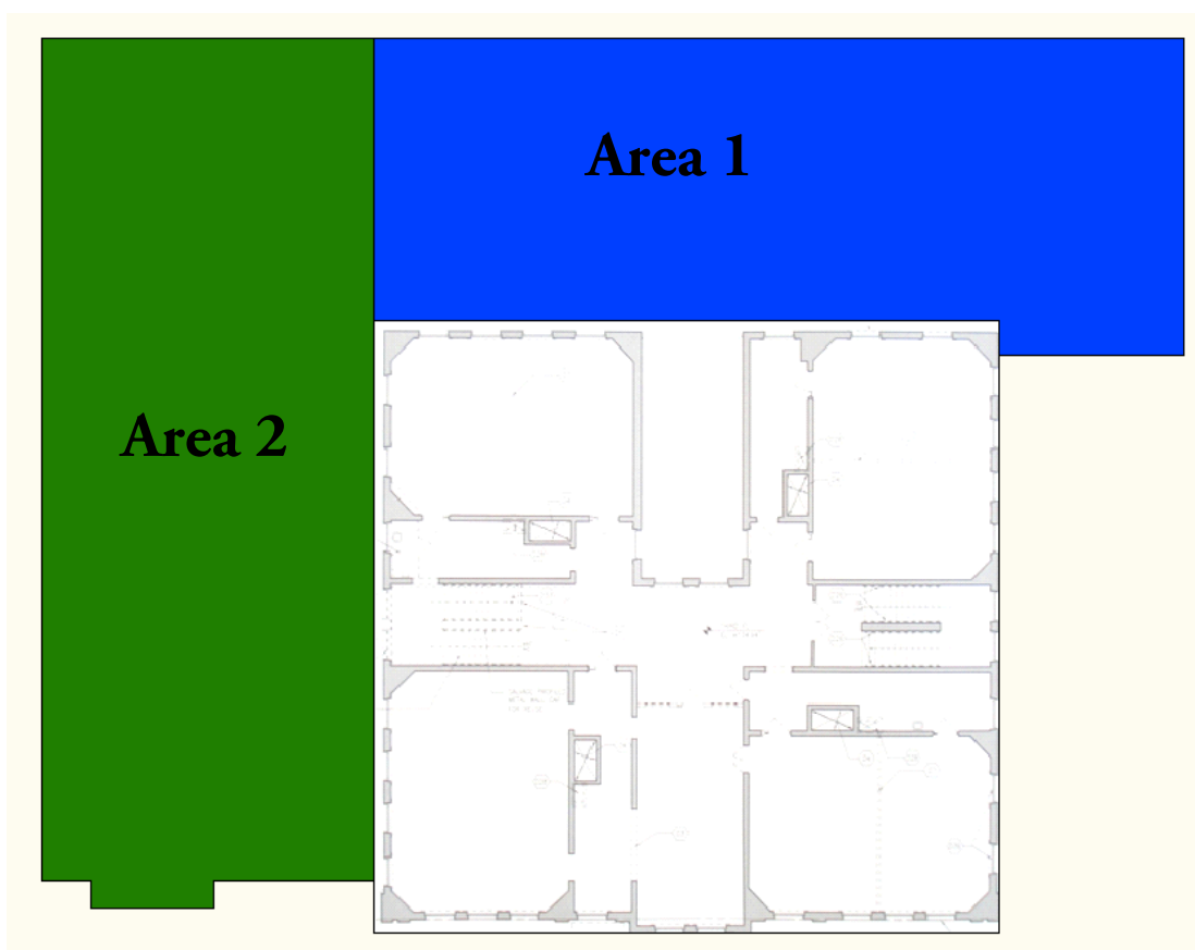
Separate Lateral Systems to the Building (Figure 11)
